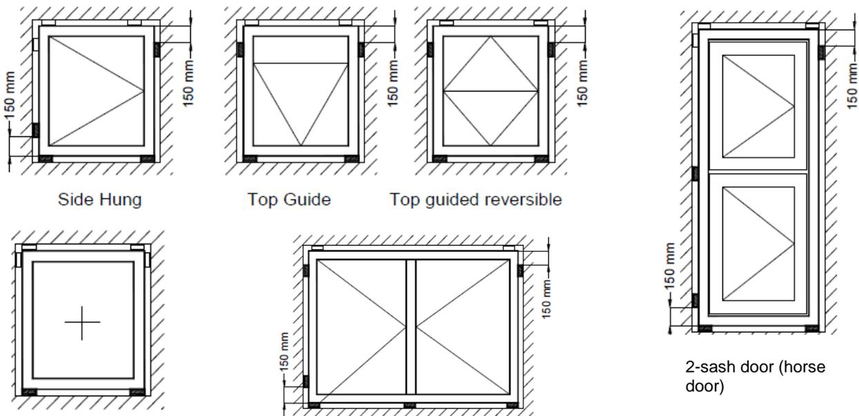
**Fig. 5. Basic arrangement of support points for EURO windows**
