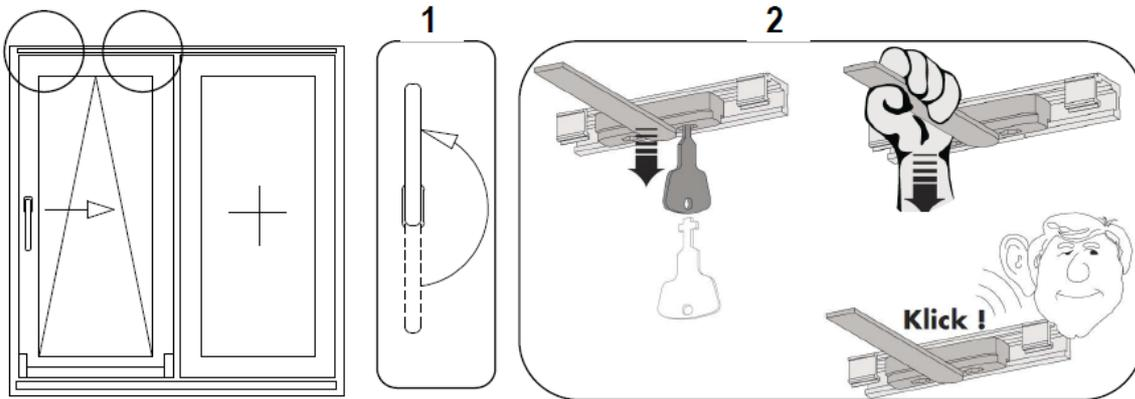
**Fig. 19 Removing tilt-and-slide sash**
