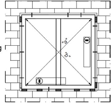
**Fig. 4. Checking the window frame setting in the wall opening**
