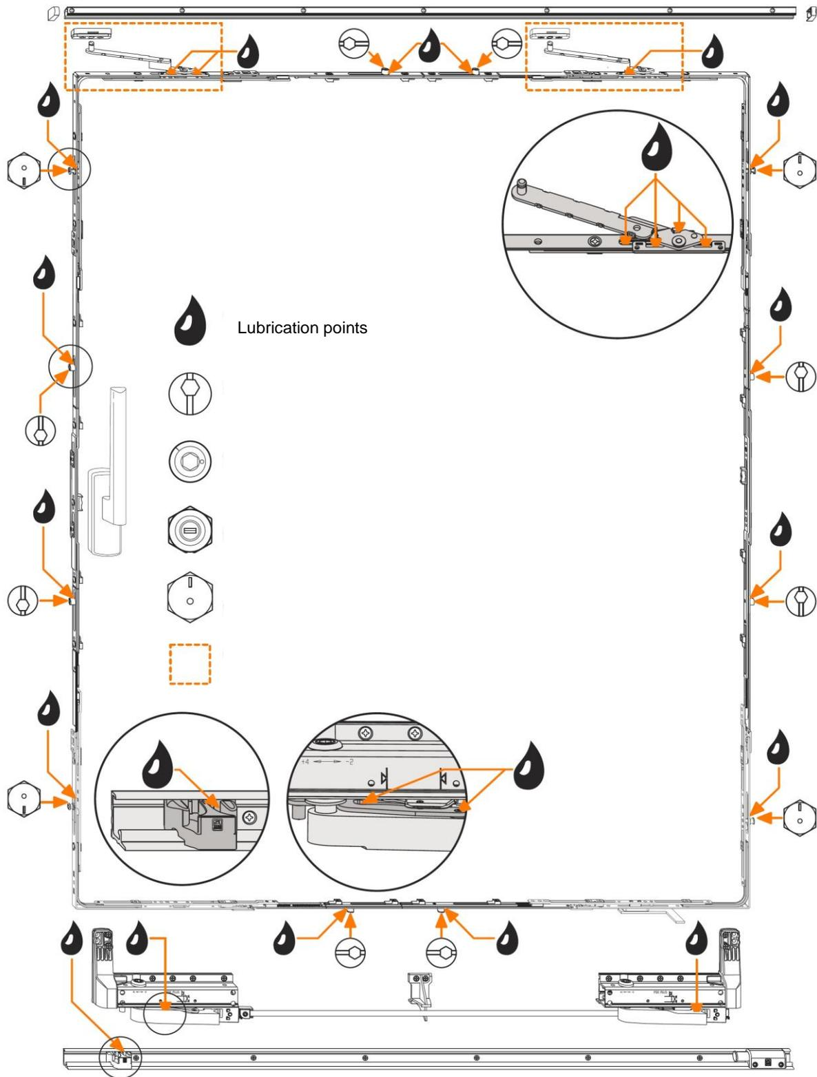
**Fig. 20** Lubrication of fittings in tilt and slide sash (lubricants without acid and resin spray are recommended)
