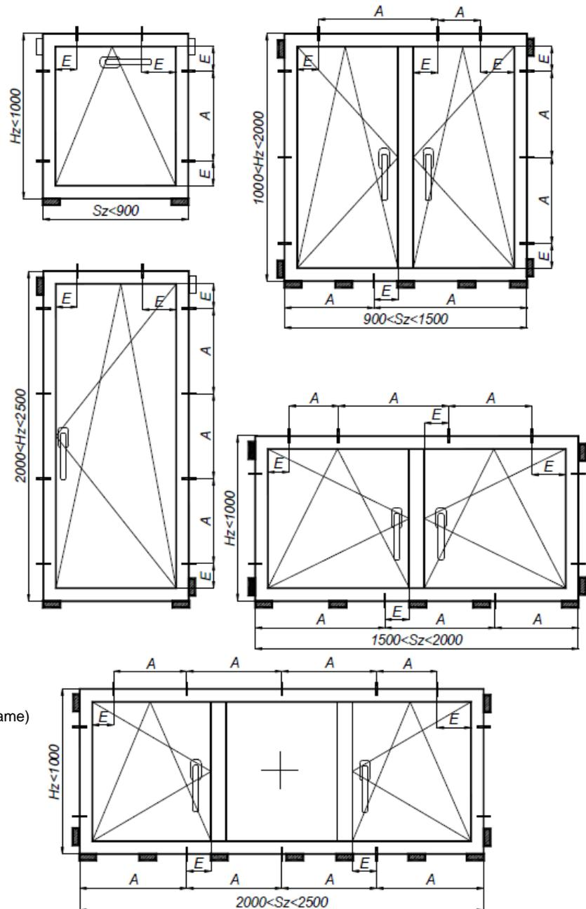
**Fig. 3 Window support and fixing points**
