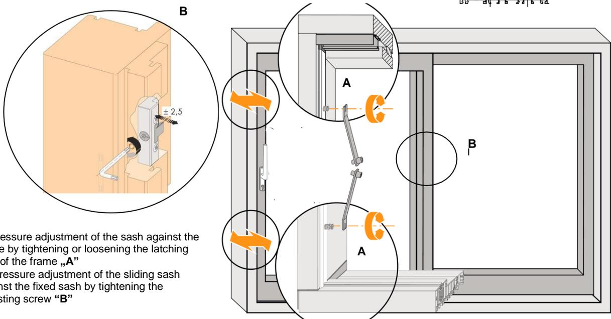
1. Pressure adjustment of the sash against the frame by tightening or loosening the latching pins of the frame „A”
