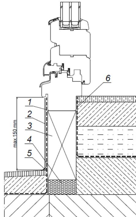
**Fig. 13 Sealing of the balcony door**
