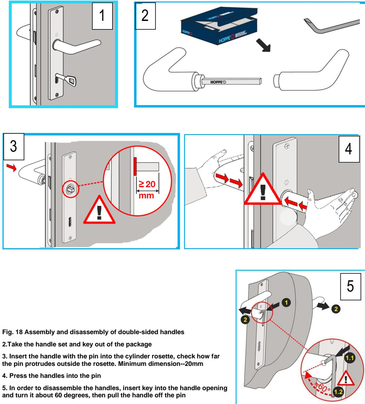
**Fig. 18 Assembly and disassembly of double-sided handles**
