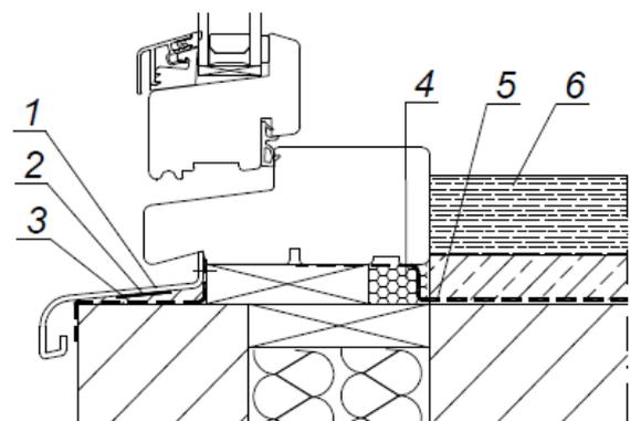
**Fig. 11. Example of fitting exterior and interior window sill (Euro windows)**
