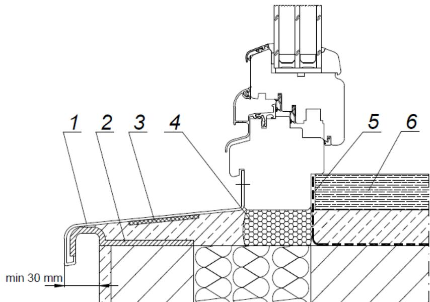
**Fig. 10. Example of fitting exterior and interior window sill**
