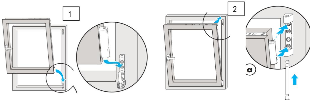
**Fig. 15. Installing the sashes**
