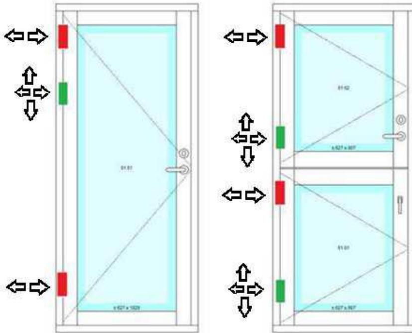
**■ Hinge with horizontal and vertical adjustment**
