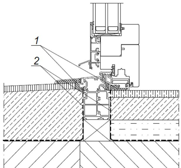
**Fig. 14. Sealing of the balcony door with aluminium threshold**
