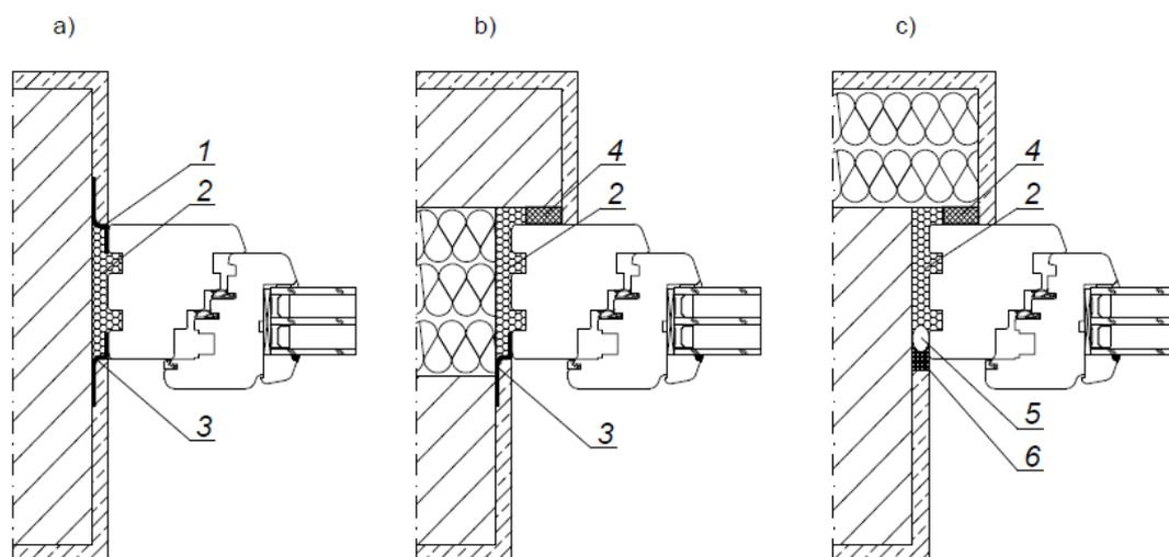
**Fig. 9. Window sealing depending on the wall structure**
