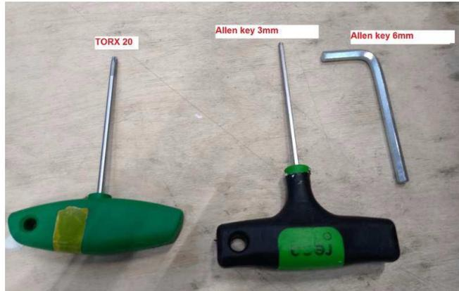
**IMPORTANT! The adjustment of the adjustable hinges with using of CRANKED KEYS is forbidden, because of big risk to damage the hinges!**
