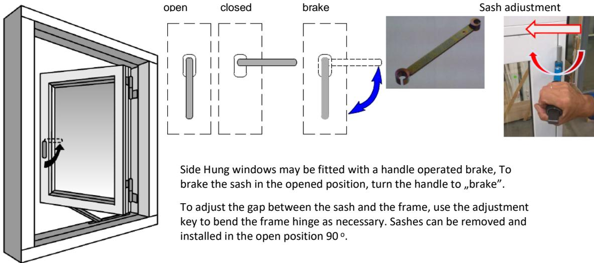
Side Hung windows may be fitted with a handle operated brake, To brake the sash in the opened position, turn the handle to „brake”.
