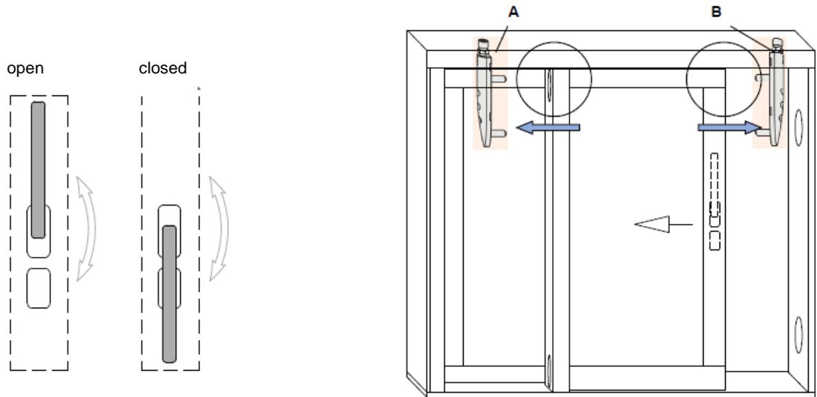
**Fig. 23 Removing the leaves**
