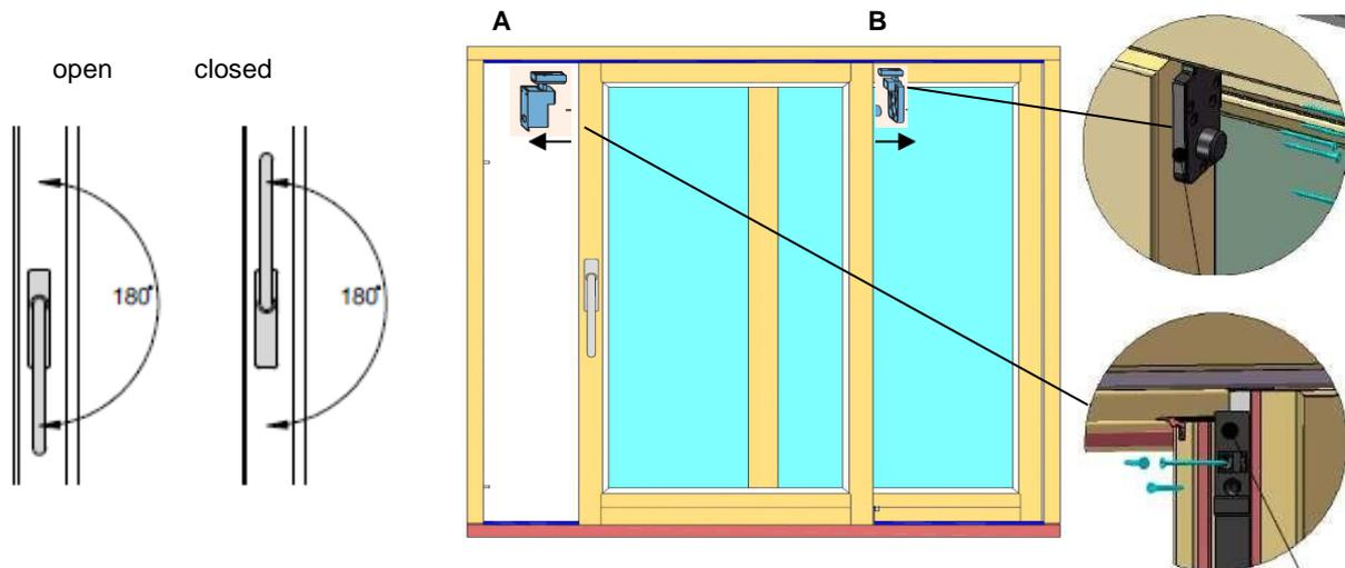
**Fig. 21 Removing the sashes**
