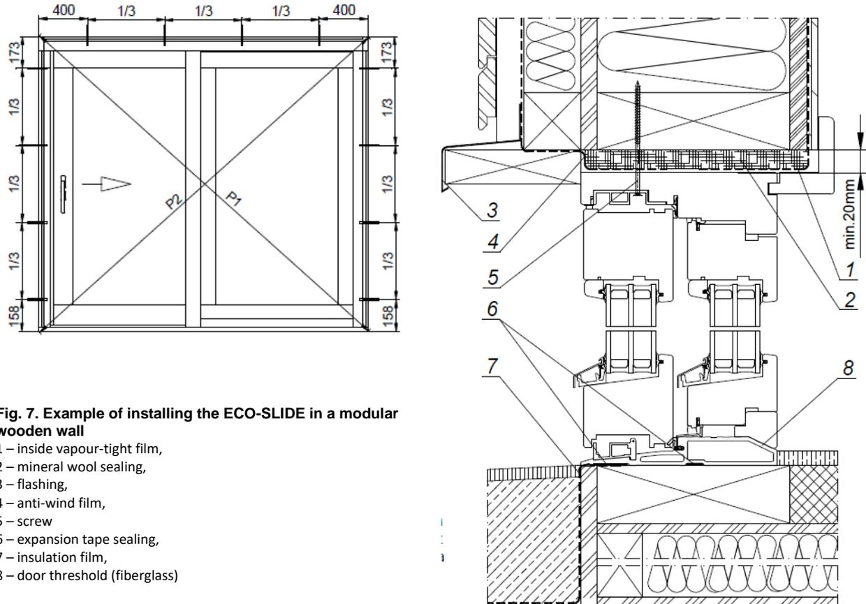
**Fig. 7. Example of installing the ECO-SLIDE in a modular wooden wall**
