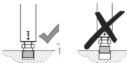
Adjust the overlap of the active sash slides by tightening or loosening the adjustment screws
